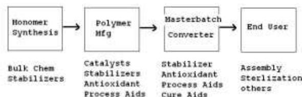
Figure 2. Process chain where additives occur
